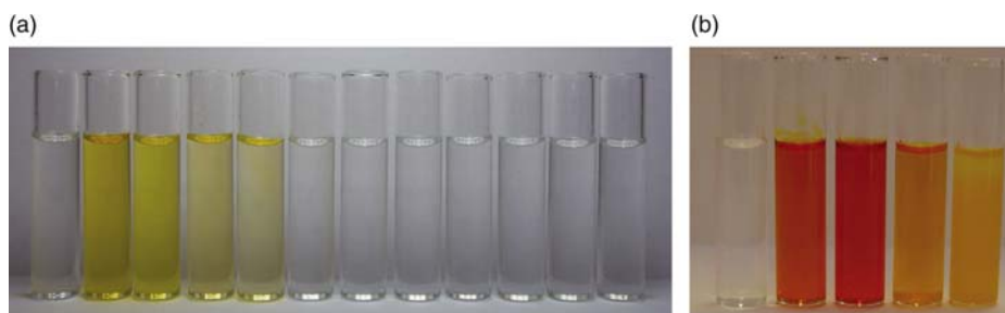
Figure 2. Photograph of M3 solutions in DMSO ( [\text{M3}] = 2 \times 10^{-3} \text{ M} ). (a) Upon addition of complexing anions, from left to right: control blank, acetate, benzoate, oxalate, p -toluenesulphonate, chloroacetate, dihydrogen phosphate, trifluoroacetate, bromide, methanesulphonate, chloride and iodide. (b) Upon addition of basic anions producing deprotonation of the urea group, from left to right: control blank, \text{OH}^- , \text{F}^- , \text{HCO}_3^- and \text{PO}_4^{3-} .
